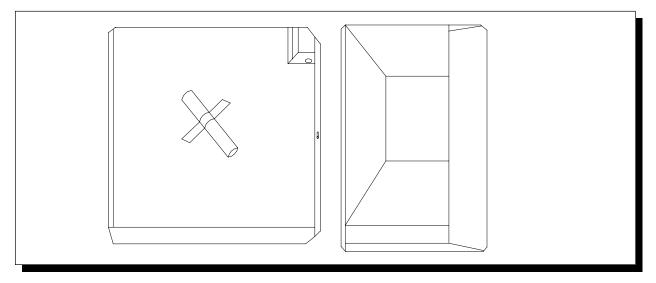
6. Install gasketing on top of bin if required. Gasket material must be positioned so that it extends to the outside edge of the perimeter of the cuber chassis when the cuber is in place.
